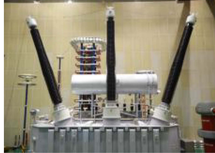
550kV OIP Bushings
