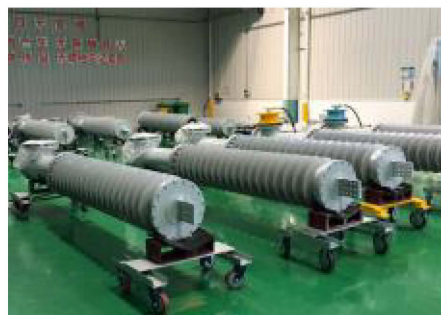
GIS/GCB SF 6 Outlet Bushings
