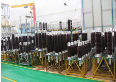
72.5-252kV OIP Bushings
