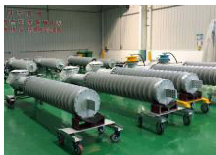
GIS/GCB SF 6 Outlet Bushings
