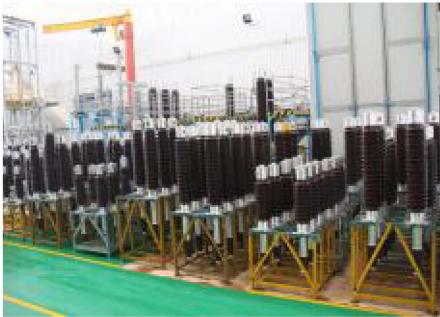
72.5-252kV OIP Bushings
